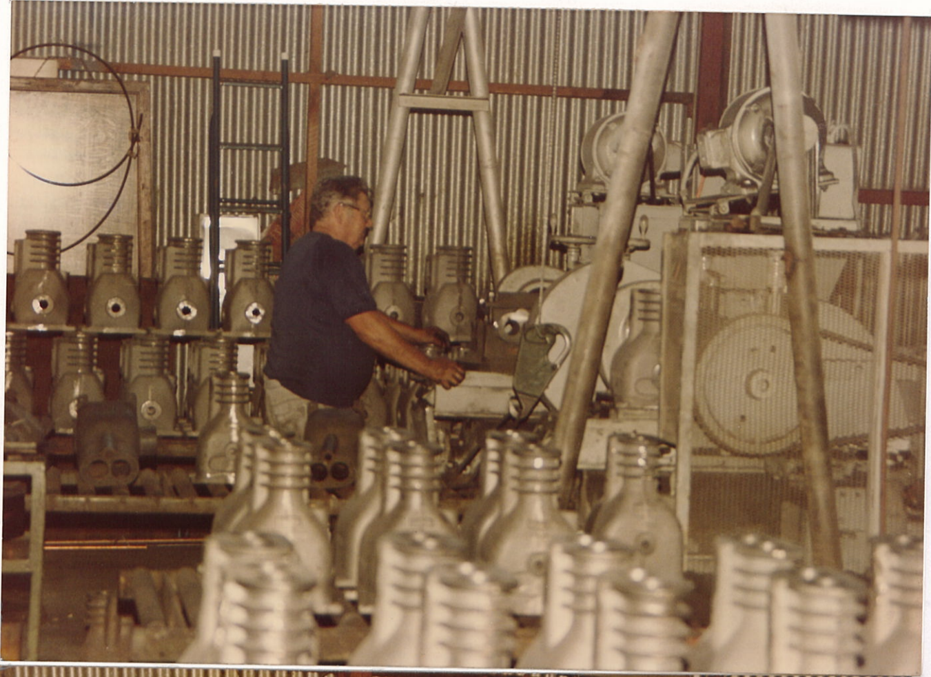
From the casting to the complete refrigerator. Unmachined pistons, cylinder heads, front covers and valve plates.
