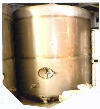
DIAMETER 2900MM X VERTICAL WALL HEIGHT 2800MM.MOUNTED ON APPROX.
