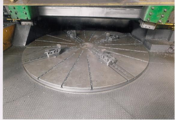
SHEET NUMBER 28058 VERTICAL BORER AND TURNING MILL.BRAND K. RAFAMET---TABLE DIAMETER 3100 MM. DOUBLE COLUMN HEADS. W/- GUARDS. SPECIFICATIONS: INCLUDES LEFT AND RIGHT HAND HEADS.
